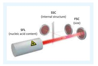
Fig. 4 Measurement principle of fluorescence flow cytometry
